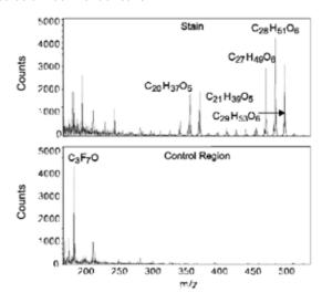
The TOF-SIMS spectrum of the droplets showing peaks in the mass range from 320-500u is shown in the top figure, while the bottom figure is from a control region on the surface. The droplets were determined to be pentaerithrytol tetraoctanoate.
