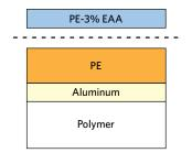
Figure 1: Schematic of PE-EAA – PE laminate showing failure location.
