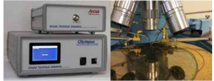
Figure 5: HBM Two Point Tester and Probe Station
