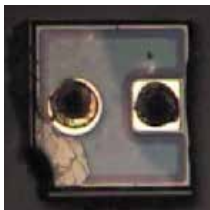
Sample surface after depackaging Die size: 300 x 300mm
