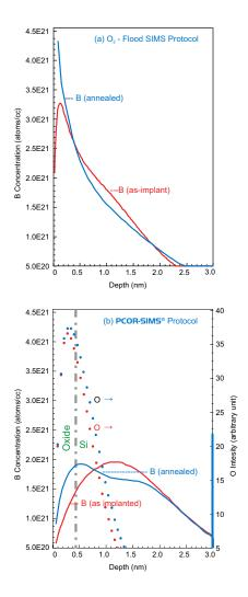
Comparison of two SIMS analysis protocols for 250eV boron implant characterization before and after anneal. Please note that concentration axes are linear unlike the usual log scales. PCOR-SIMS<sup>SM</sup> analysis of annealed B implantation detects accumulation at oxide/Si interface as expected (b). Whereas  $O_2$ -flood SIMS protocol results in un-realistic profile shapes (a).
