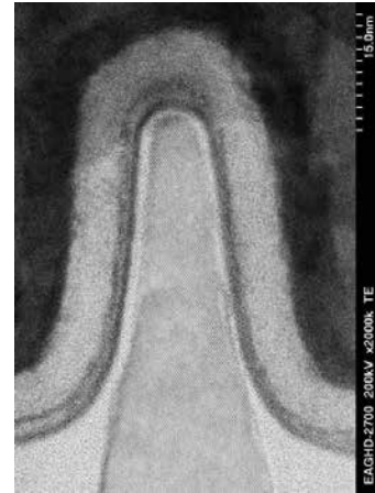
Above is a high resolution BF STEM image and below is an associated composite elemental map showing the structure of a FinFET device with single-nm scale process layers.
