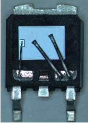
DECAP OF DEVICE WITH AL BOND WIRES
