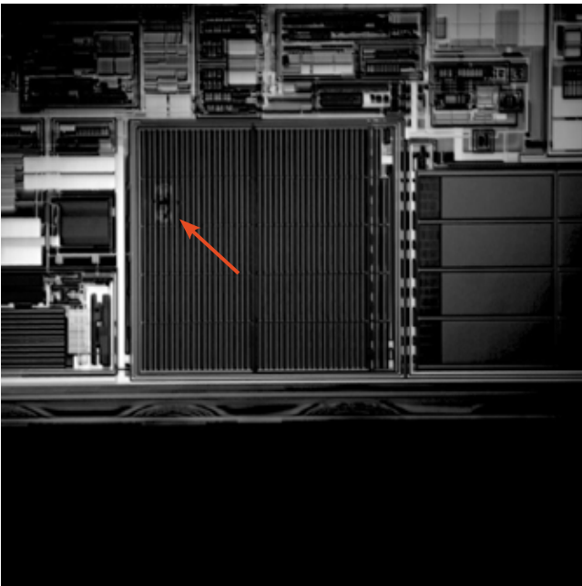
LSM – SAME DEVICE AS ABOVE (SHOWING DEFECT)
