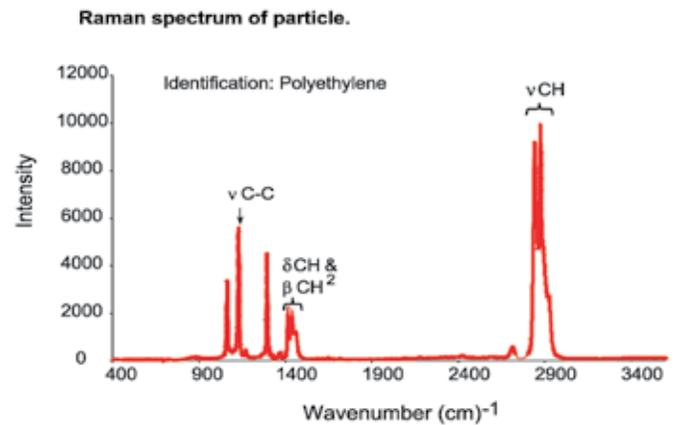
The spectrum obtained from the particle matched a reference spectrum of polyethylene. The high spatial resolution of Raman Spectroscopy makes it ideal to investigate particles in the 1 $\mu$ m size range. It is especially useful in combination with SEM-EDS to determine the elemental species present.
