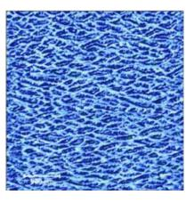
Figure 4: Strained, then etched 3 minutes
