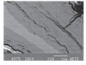
SEM micrograph obtained at the weld area, showing porosity, cracks and particles in the scale 20X.
