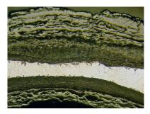
Optical micrograph of corroded steel pipe showing intergranular attack and reduced thickness 16X.
