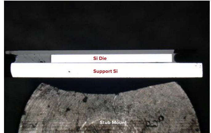
Figure 2: Mechanical x-section across whole die: side view of Figure 1 sectioned to the red line.
