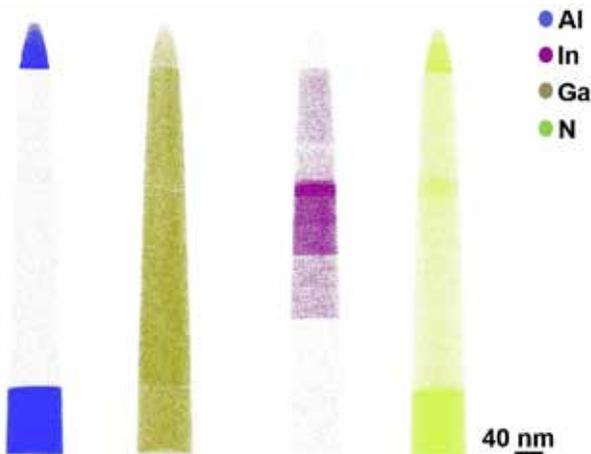
**2. Compositional Variation:** APT provides multiples ways to analyze composition, such as line profile, proxigram and iso-concentration surfaces that are based on depth or concentration.
