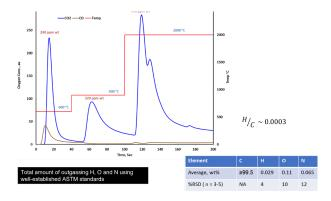
**Figure 3:** The plot shows oxygen concentration in composite is compared with heating time and temperature. The table shows average Concentration and RSD values of carbon, hydrogen, oxygen, and nitrogen.
