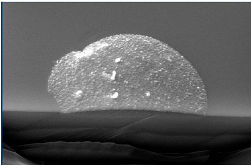
Figure 4a: SEM image of the FIB cross-sectioned bubble defect.
