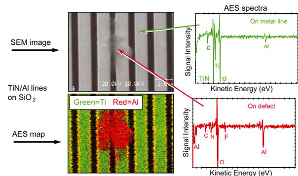
Figure 2: Auger analysis shows the thin residue is an Al flake, probably originating from the etch chamber.
