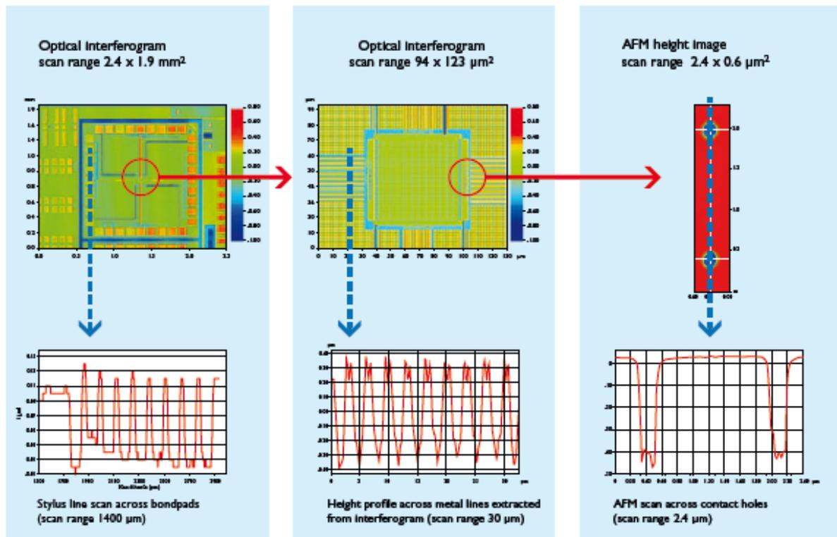
Fig. 1: Example of a mounted chip where the three different surface profile techniques were used to characterize specific parts of the device on a scale ranging from mm to nm.
