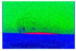
Green=W Red=C Blue=Si Figure 4b: Auger map of the bubble defect after in-situ FIB cross-sectioning.
