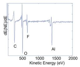
Figure 3a: Normal Chip Auger Spectrum of Bond Pad
