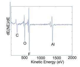
Figure 3b: Contaminated Chip Auger Spectrum of Bond Pad
