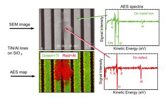
Figure 2: Auger analysis shows the thin residue is an Al flake, probably originating from the etch chamber.
