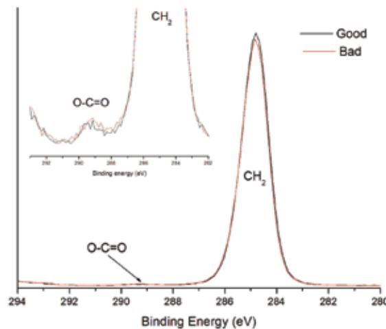
**Figure 2:** High resolution photoemission spectra of good and bad heat seal surface. Inset shows weak  $\text{O}-\text{C}=\text{O}$  expected for EAA.
