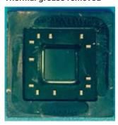
Typically looking for corrosion, discoloration of the substrate, cracking or chip outs on the die
