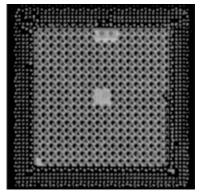
Typically looking for small delamination areas, heat spreader glue adhesion gaps and thermal grease attach area
