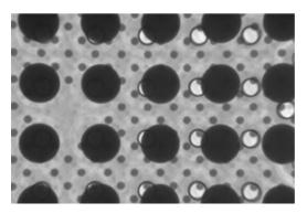
Typically looking for void growth in the solder bumps/balls, or deformation
