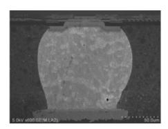
Typically looking for small cracking of the solder, intermetallic thickness, voiding/delamination in the weave or along the vias.
