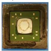
Thermal grease removed
