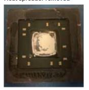
Thermal grease removed
