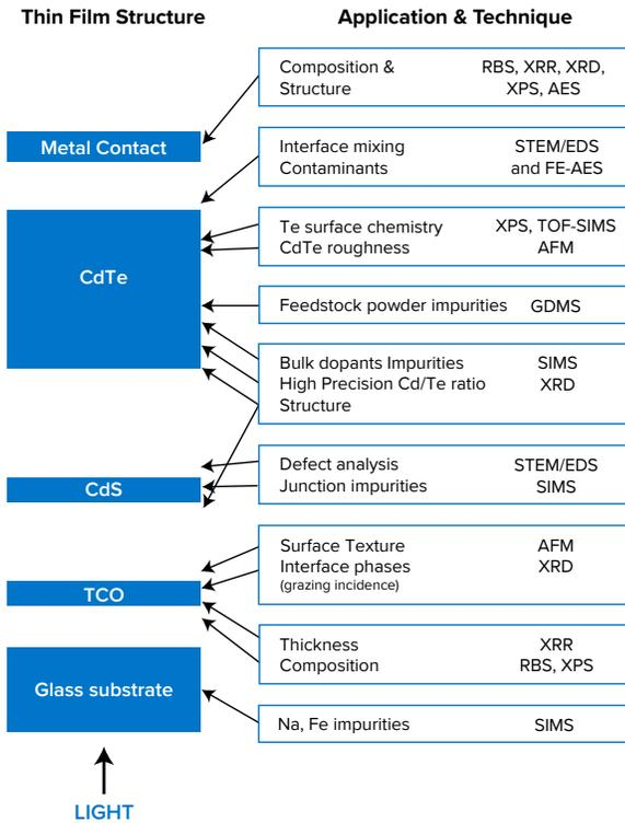
CdTe thin film PV is one of the main thin film PV technologies being commercialized. CdTe has the advantage of a direct bandgap which matches well with the solar spectrum, a high absorption coefficient, the ability to be doped both n-type and p-type, and processes that can work for low cost, large scale manufacturing.
