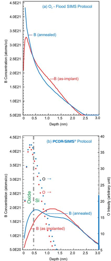
Comparison of two SIMS analysis protocols for 250eV boron implant characterization before and after anneal. Please note that concentration axes are linear unlike the usual log scales. PCOR-SIMS<sup>SM</sup> analysis of annealed B implantation detects accumulation at oxide/Si interface as expected (b). Whereas O<sub>2</sub>-flood SIMS protocol results in un-realistic profile shapes (a).
