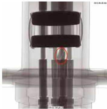
Radiograph of a bent contact pin inside a connector
