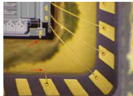
Fused open bond wire inside an integrated circuit
