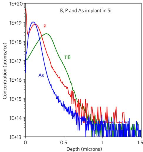
Profiles of B, P and As implant standards in Si. These standards are calibrated with NIST SRM. SIMS profiles provide accurate doping concentrations vs. depth, with excellent detection sensitivity and dynamic range.
