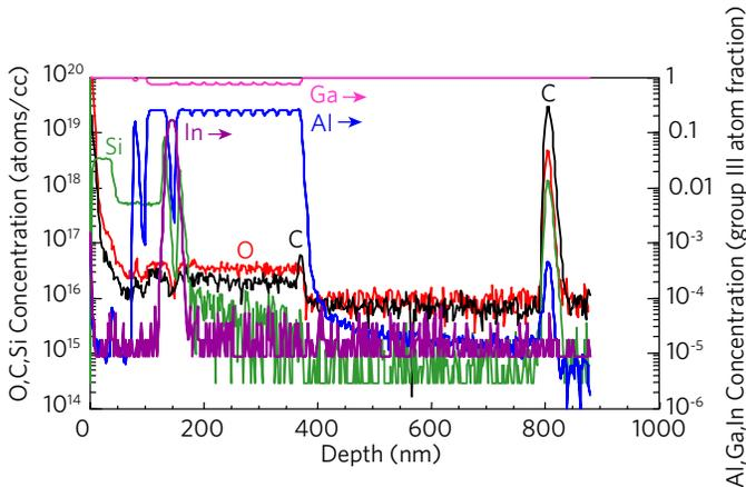
Compound (III-V) semiconductor device characterization, complete with composition and dopant/impurity concentration quantification. The profile is optimized for C and O impurity detection and for good depth resolution.
