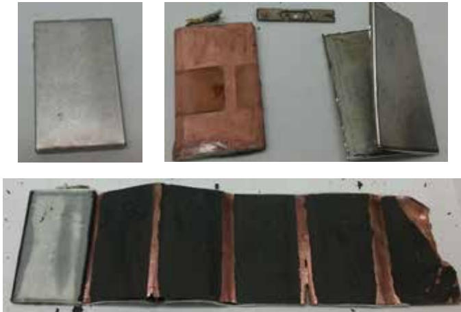
Figure 7: Disassembled battery. (Source: EAG Laboratories)
