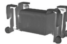
Reconstruction of a 4mm long inductor package
