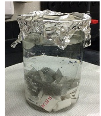
Figure 2. Stainless steel screen and sectioned PVC pipe substrates soaking in dilution water. Substrates soaked for >24 hours prior to use in trial.
