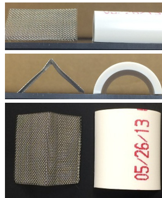
Figure 1. Side view, front view, and top-down view of the bent stainless steel screen “tent” (left) and the sectioned PVC pipe substrates (right).
