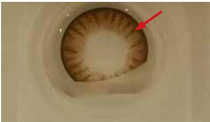
**Figure 1a.** This optical image shows the top view of a lens examined in this study. The red arrow indicates where the lens was sectioned for SEM analysis using a cryo-microtome with a diamond blade.
