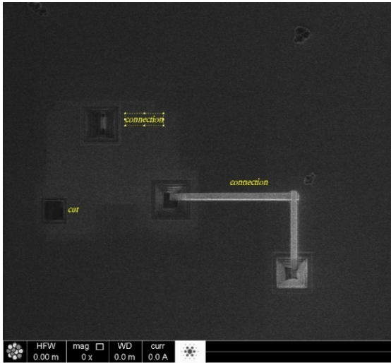
Figure 10: The actual cuts and jumper are laid
