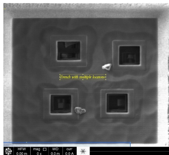
Figure 9: Four smaller windows are created in the areas where the editing is to be performed.
