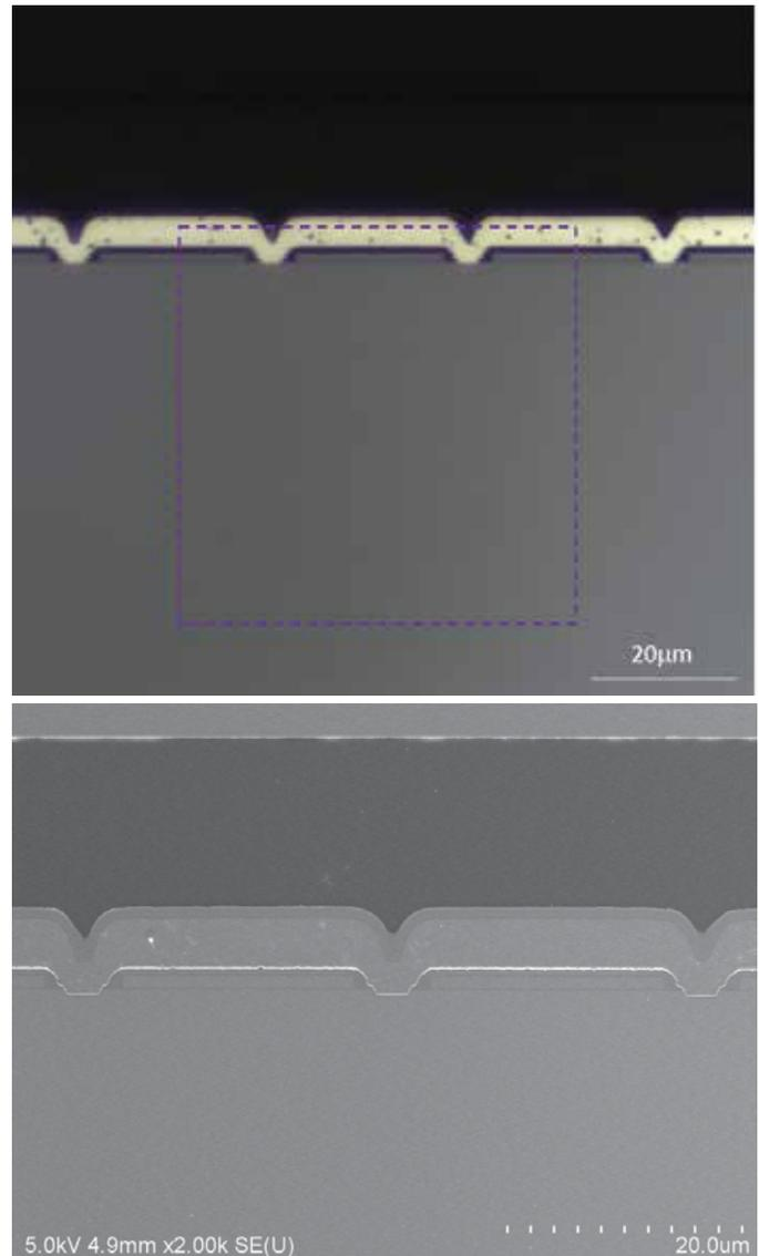
**Figure 2: Optical microscopy image (top) and SEM image (bottom) of the prepared cross-section. The purple square indicates the analysis area for the 50µm x 50µm SCM images.**
