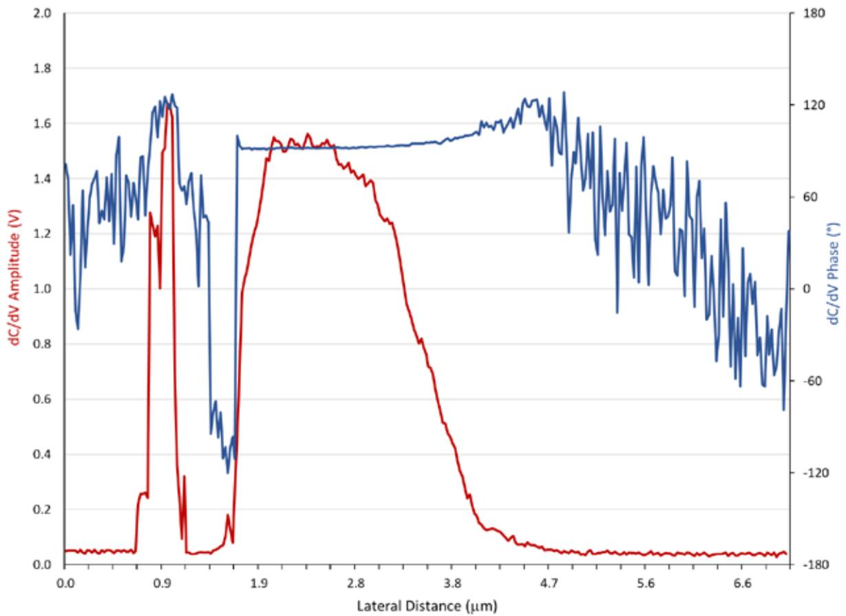
Figure 7: Representative doping profiles taken along the black arrow in the SCM Data image. The red trace is dC/dV amplitude (relative doping levels) and the blue trace is dC/dV phase (relative doping type)
