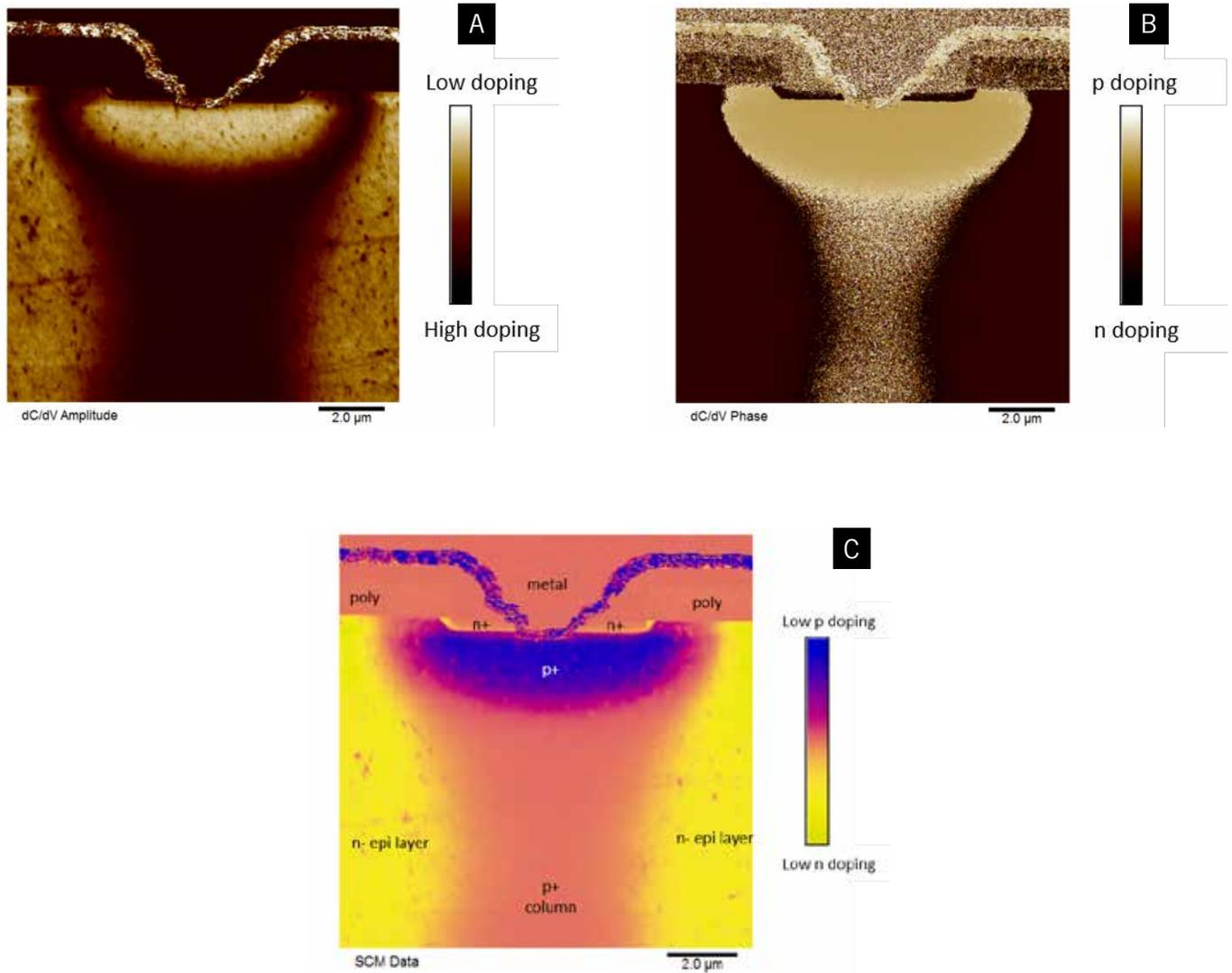
Figure 6: SCM images of the cross-sectioned MOSFET (A)  $dc/dV$  amplitude (relative dopant levels), (B)  $dC/dV$  phase (dopant type), (C) SCM data image (15  $\mu\text{m}$  x 15  $\mu\text{m}$ )
