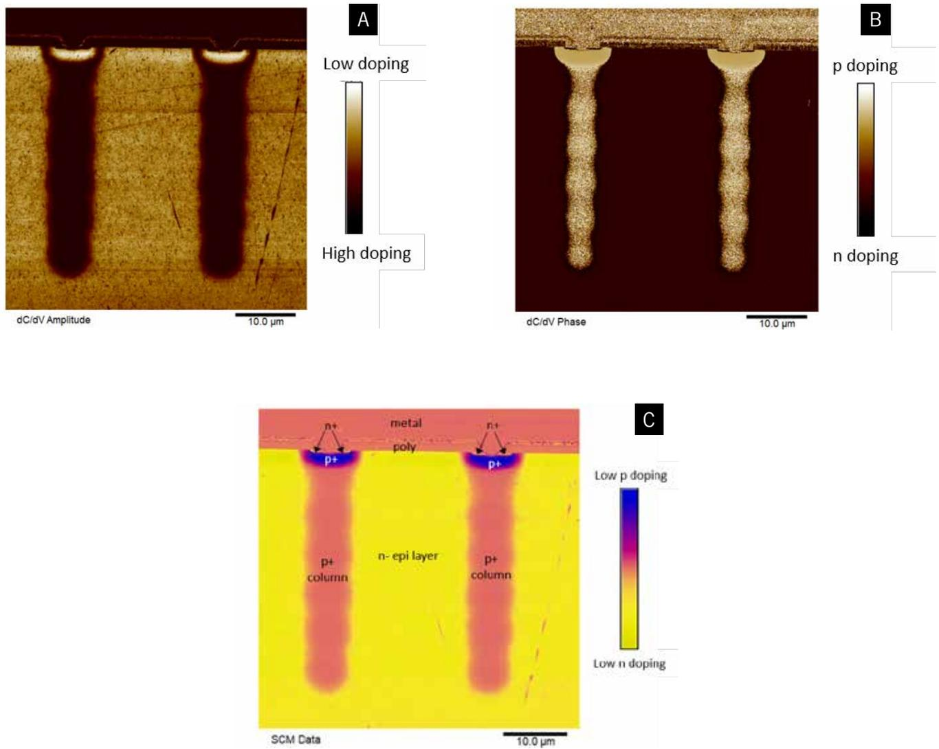
Figure 4: SCM images of the cross-sectioned MOSFET (A) dc/dV amplitude (relative dopant levels, bright = low doping), (B) dC/dV phase (dopant type, brown = n type, white = p type), (C) Combined SCM data image (50μm x 50μm)
