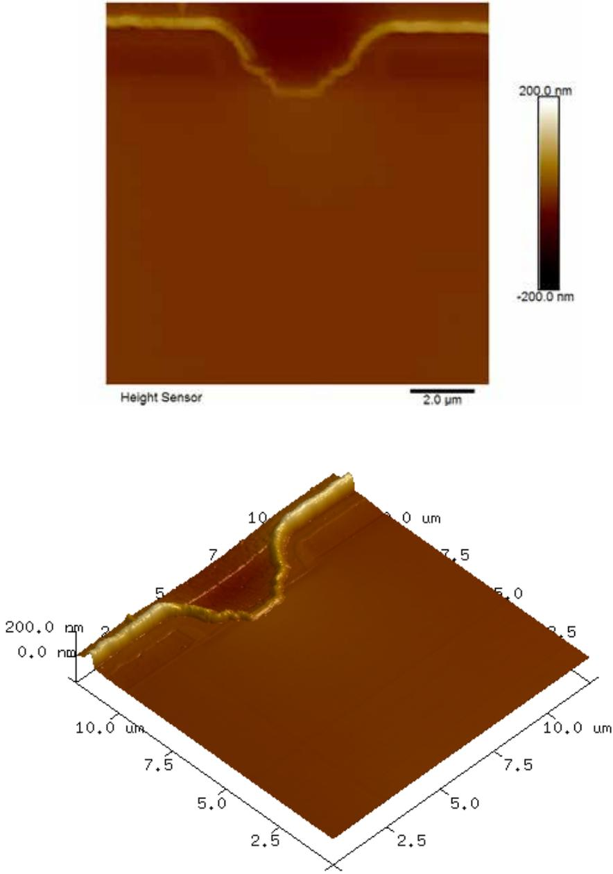
Figure 5: AFM height images of the cross-sectioned MOSFET (15μm x 15μm x 400nm)
