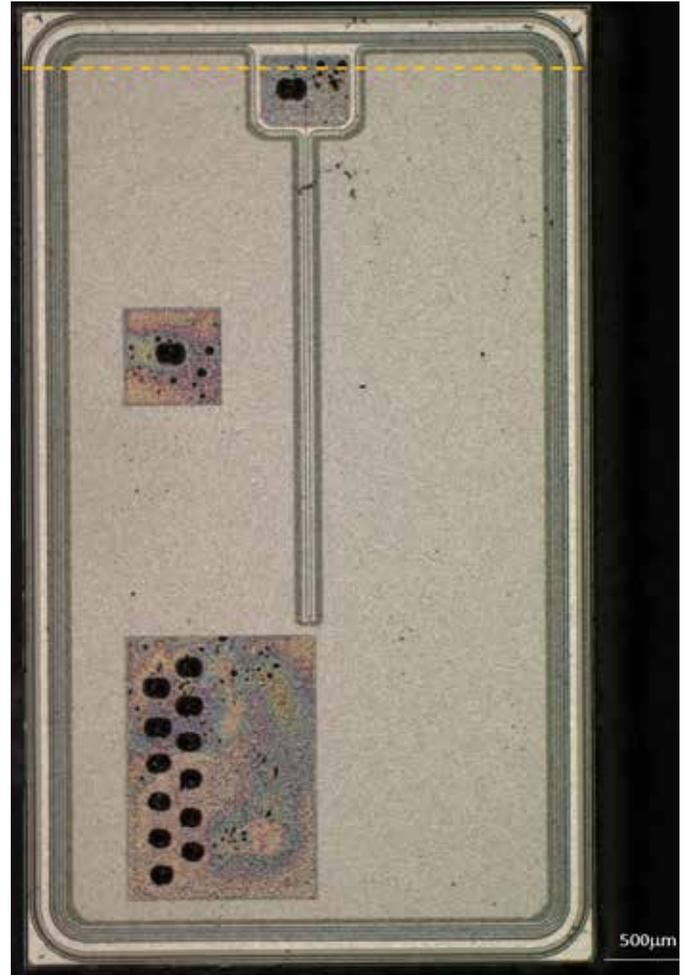
**Figure 1: Top-down optical microscopy view of the depackaged die. The dotted orange line shows the plane that was cross-sectioned.**
