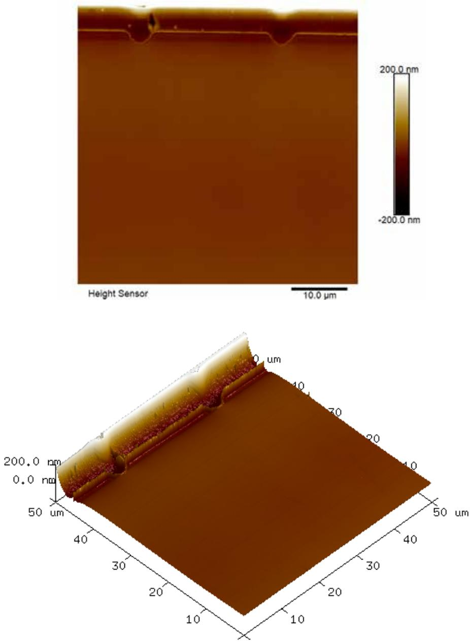
Figure 3: AFM height images of the cross-sectioned MOSFET (50μm x 50μm x 400nm)
