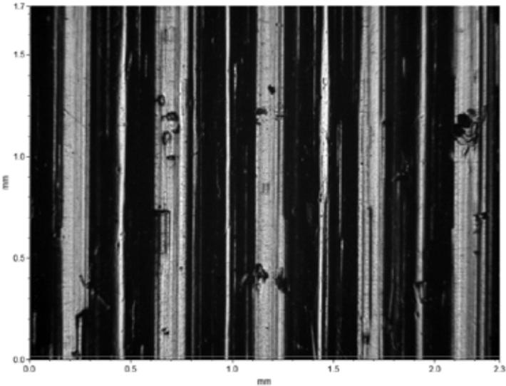
Figure 7: Turning, 6.3μm R<sub>a</sub>
