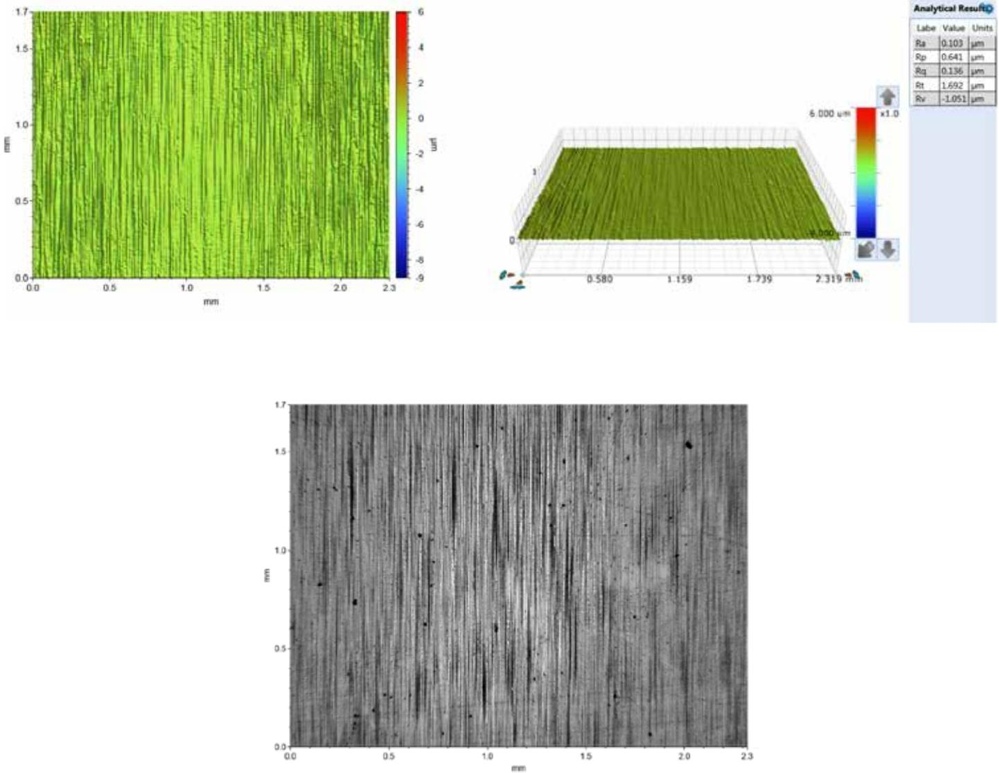
Figure 2: Grinding, 0.1µm  $R_a$
