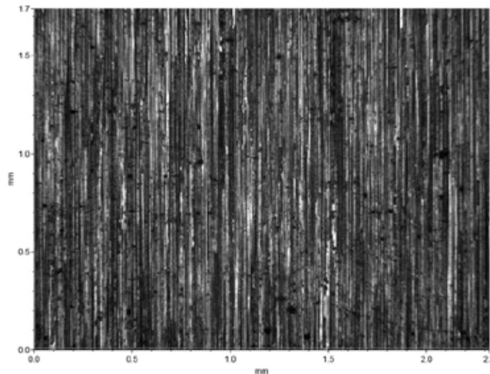
**Figure 3: Grinding, 0.8µm R<sub>a</sub>**
