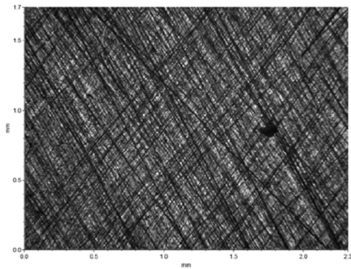
Figure 4: Flat lapping,  $0.2\mu\text{m } R_a$
