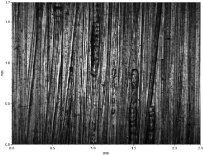
Figure 5: Reaming, 0.8µm Ra
