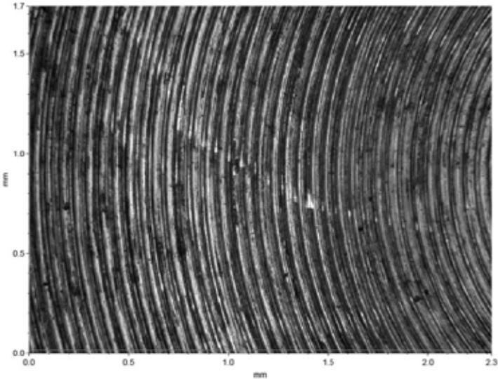
Figure 10: Flange face, 0.614µm R<sub>a</sub>
