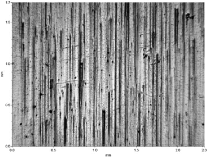
Figure 6: Turning, 0.8μm Ra
