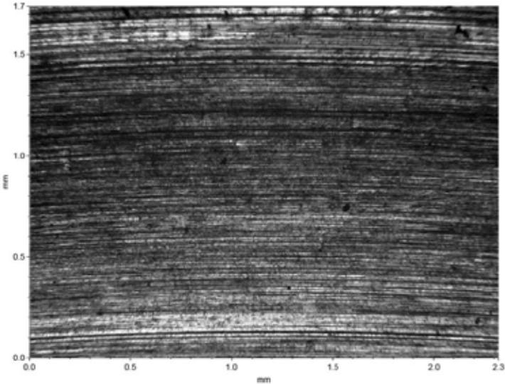
Figure 11: Flange sealing surface, 0.219μm R<sub>a</sub>
