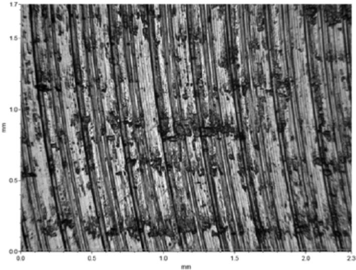
Figure 9: Vertical Milling, 0.8μm Ra
