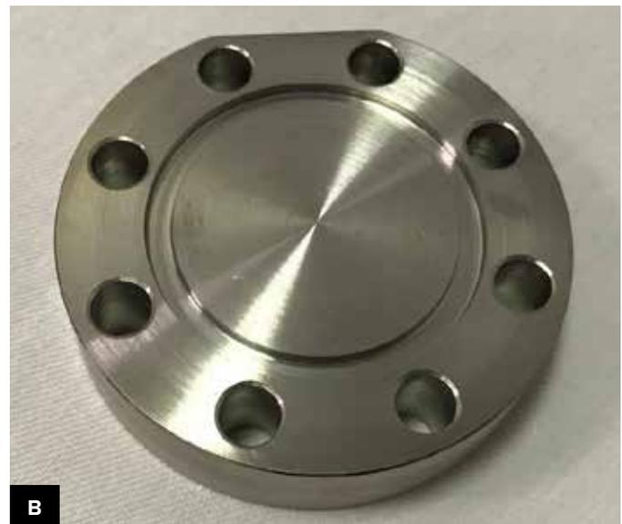
**Figure 1: Photographs of (A) the reference metal coupons (Flexbar, Islandia, New York, USA) and (B) the vacuum flange**
