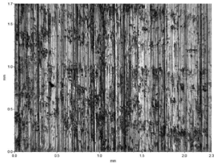
Figure 8: Horizontal Milling,  $0.8\mu\text{m } R_a$
