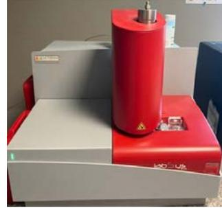
Figure 12 : Instrument Setaram LABSYS evo
