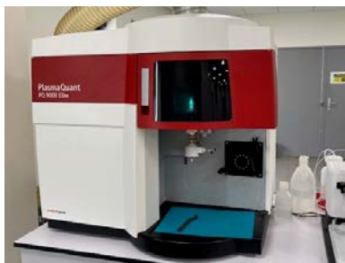
Figure 15: Analytik Jena PQ9000 instrument
