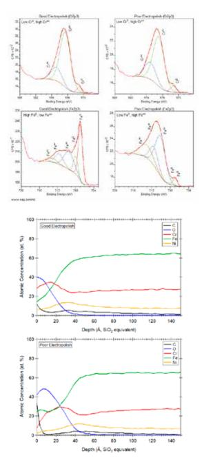
enrichment using the Cr<sup>metallic</sup>/Fe<sup>metallic</sup> and Cr<sup>ox</sup>/ Fe<sup>ox</sup> ratios obtained by XPS. The passivation layer structure, encompassing the chromium-enriched oxide thickness, surface carbon layer thickness, detached iron oxide layer thickness, metal oxide layer thickness, and Cr/Fe ratios as a function of depth, is measured by AES.
