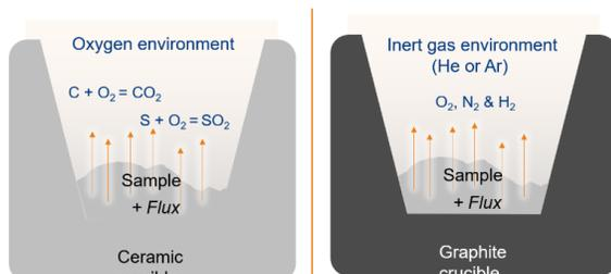
**Figure 1:** Carbon and sulfur are measured based on combustion method for gas extraction (left). Oxygen, nitrogen, and hydrogen are measured using inert gas fusion gas extraction method (right).
