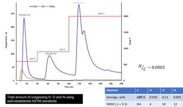
**Figure 3:** The plot shows oxygen concentration in composite is compared with heating time and temperature. The table shows average Concentration and RSD values of carbon, hydrogen, oxygen, and nitrogen.
