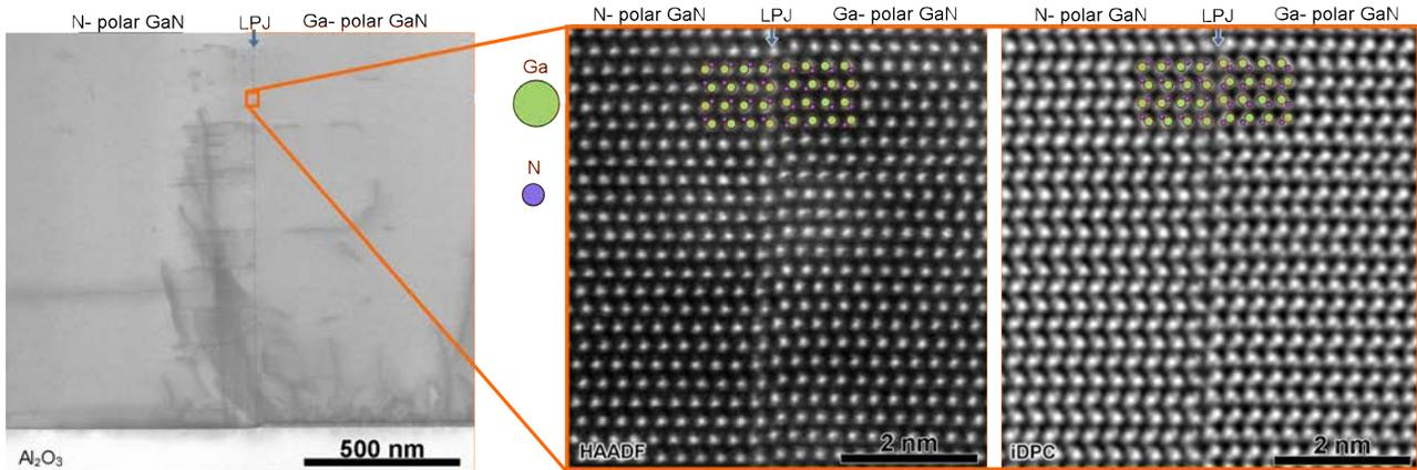
Figure 2: A LPJ GaN sample with the overview shown on the left side. The IDB is indicated by the blue arrow. The two images on the right outlined in orange show the high magnification atomic resolution image from the LPJ.
