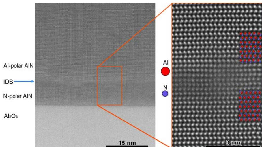
Figure 1: Al-polar AlN film grown on a sapphire substrate using a N-polar AlN buffer layer. The left image shows the overview of the structure with the inversion boundary noted by the 'IDB' text and blue line. The right shows the atomic resolution HAADF image with atom column schematic overlaid on the image.
