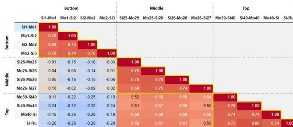
Figure 4: The correlation matrix between the roughness profiles of different interfaces within the multilayer stack. Values close to +1 (red) indicate strong positive correlation. Values close to -1 (blue) indicate strong negative correlation. Zero indicates no correlation. Short-range correlations are highlighted in yellow.
