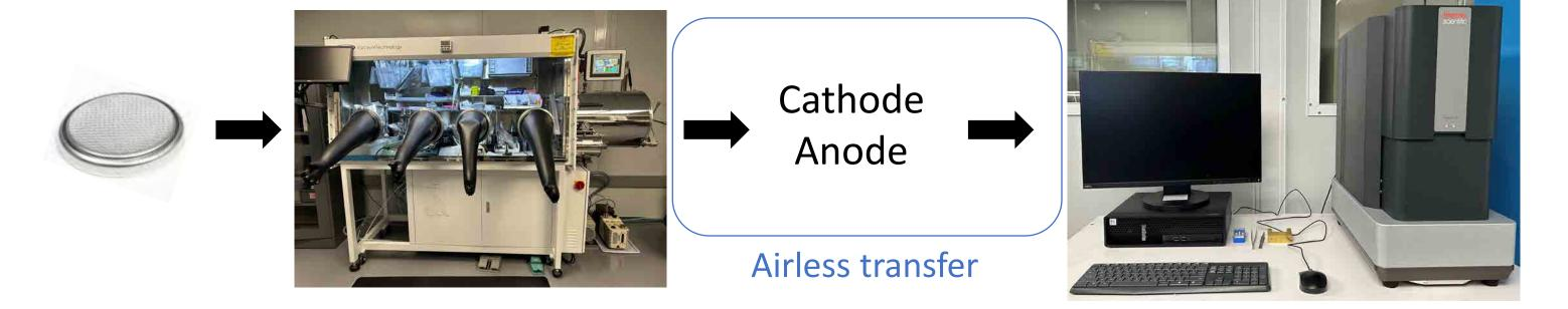
The two coin cells were disassembled in an argon glove box. Cathode and anode films were isolated from the cells and washed with dimethyl carbonate (DMC) a few times to remove electrolyte before being mounted on an airless transfer container for SEM/EDS imaging.
