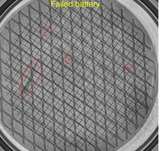
The failed battery contains lots of impurity particles.
