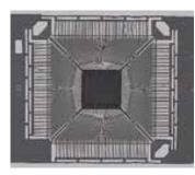
Lead frame: High dynamic range makes it easy to identify wire bonds, voids and cracks
